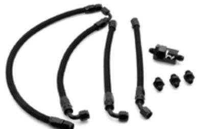
This set is designed for the return-less setup. This kit also comes with 4 lines. The first line goes from the hard line (from the fuel tank) to the FPR, the second line goes from the FPR to the other hard line (back to the fuel tank), the third line goes from the FPR to the inline fuel filter, and the final line goes from the fuel filter to the center port on the Hybrid Racing fuel rail.
